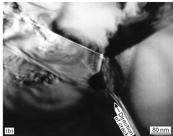
Figure 8 Fringes around (a) the crack-tips (arrowed) of the 15 vol% SiC “nanocomposite”, most probably resulting from fracture steps (Fig. 7c), and (b) the crack-tip of alumina (in the absence of dislocations the healing of the crack-tip may be incomplete). (c) Dislocation network obtained in the 15 vol% SiC “nanocomposite” at the sintering stage (this, and not a crack healing process, is the source of the dislocations in Fig. 8a).
